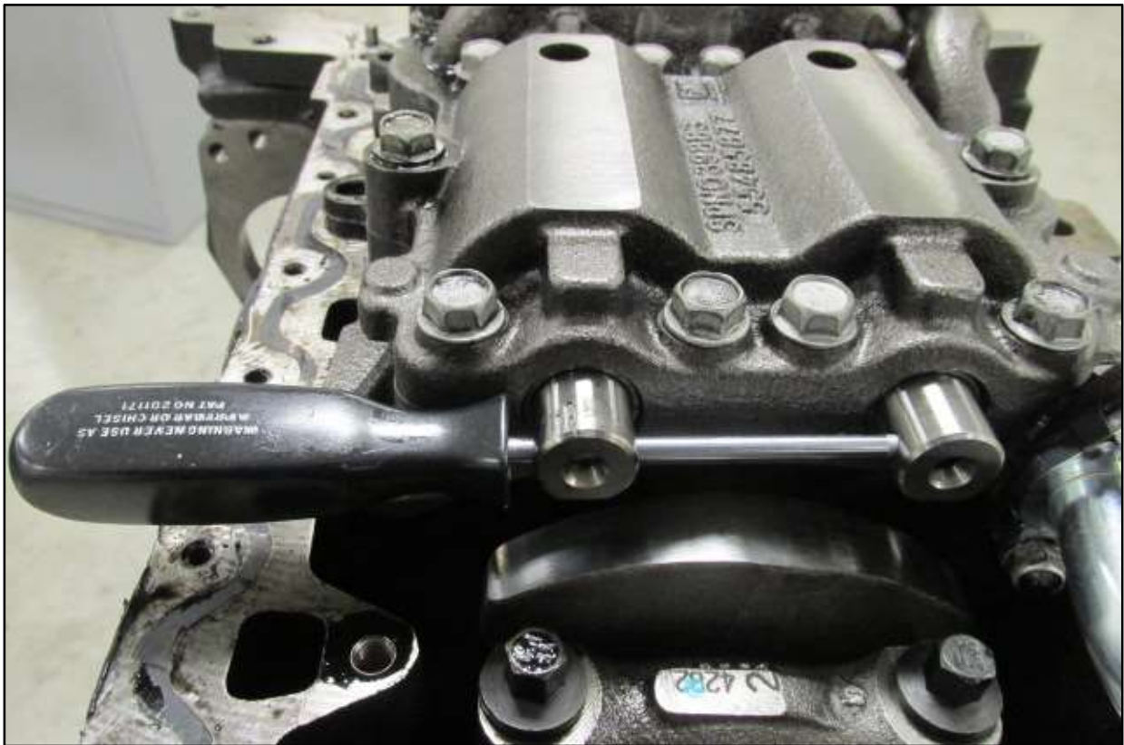
Figure 6-8, 2.8L LWN Balance Shaft Timing with Alternative Tool
