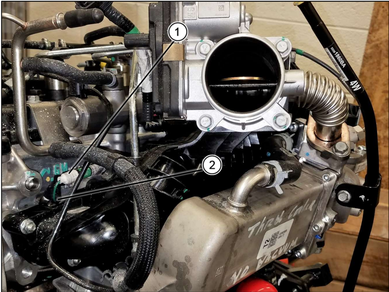
Figure 6-6, 2.8L LWN Glow Plug Location
